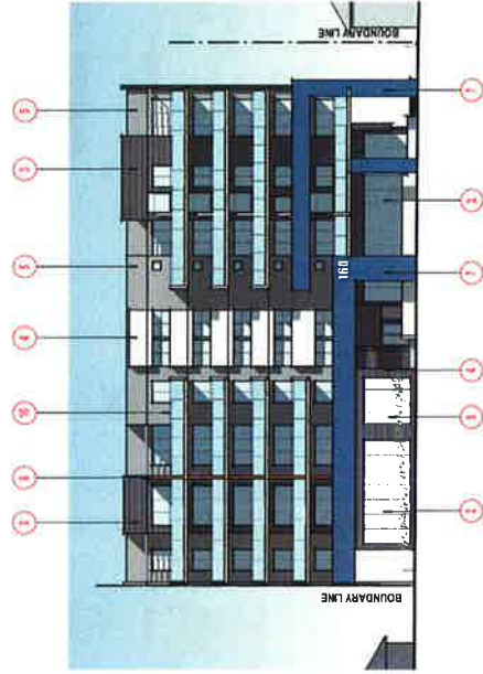
EAST ELEVATION - MATERIAL SCHEDULE
